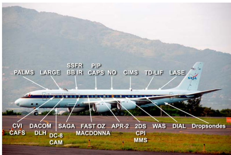
Figure 5. The NASA DC-8 showing the instruments used in TC4 and their placement on the aircraft.
