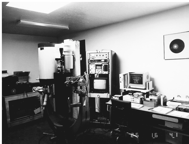
FIG. 1. Interior view of FARS showing the zenith-pointing cloud polarization lidar and coaligned midinfrared radiometer beneath the observation skylight, along with some of the computer controllers and video systems.
